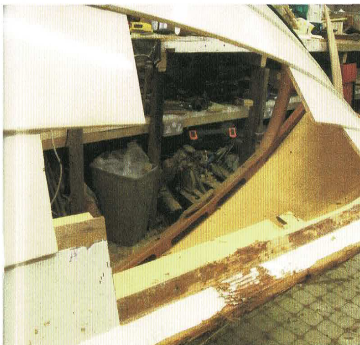
Above left: The first important stage of the repair is to remove the damaged planks carefully, which is made easier by supporting the hull on its side. Above right: With plywood graving pieces epoxied each side, the repaired plywood frame is now stronger than the original.
