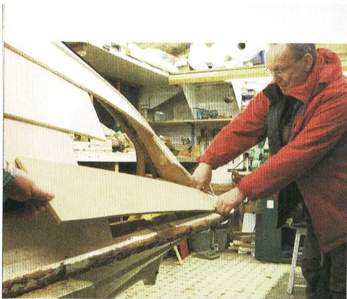
Above: Offering up the new plank. Below: Using an angle grinder to shape a new scarph in situ. Bottom: The plank in place, faired with a temporary batten until the epoxy has fully cured.
