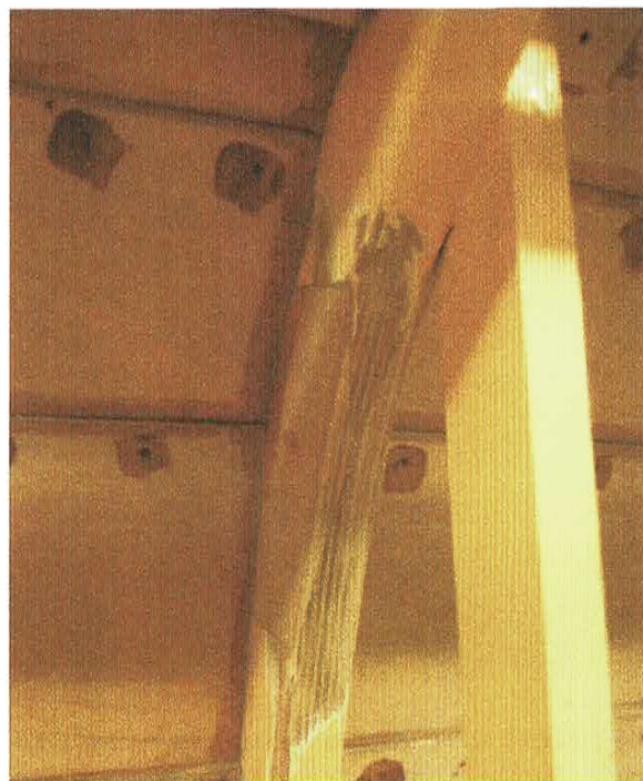
Above left: The first important stage of the repair is to remove the damaged planks carefully, which is made easier by supporting the hull on its side. Above right: With plywood graving pieces epoxied each side, the repaired plywood frame is now stronger than the original.
