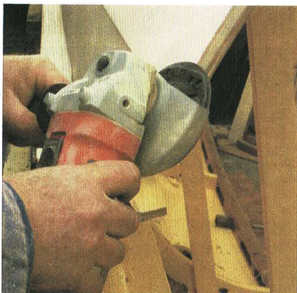
Above: Offering up the new plank. Below: Using an angle grinder to shape a new scarph in situ. Bottom: The plank in place, faired with a temporary batten until the epoxy has fully cured.
