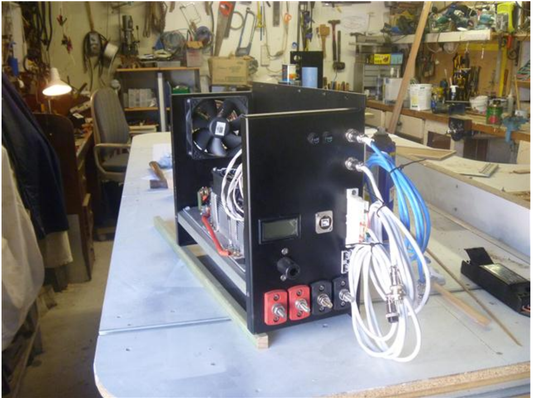
Motor control unit end view
