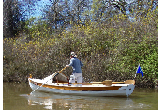
A Welsford Walkabout adapted for standup rowing with extended rowlocks
