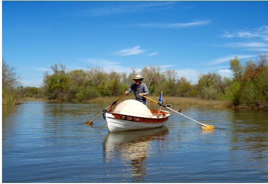
A Welsford Walkabout adapted for standup rowing with extended rowlocks
